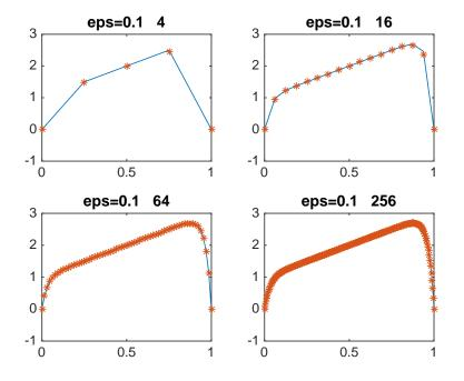
We can see in the graphs that the solution is now quite steep at each bounderies. Specifically, since we are using equi-spaced points, the scheme has some trouble resolving these regions. For example, for N = 16 we see there are only 2 points in the boundary layer region.
