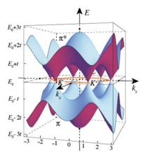
This picture is the band structure graphene, an amazing new material. Notice the six points where the levels touch. Here is a common type of diagram.
