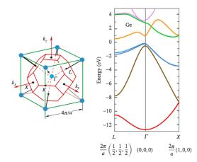
On the left is the Brillouin zone, with special points labelled. On the right are spectra along straight line paths between special points.
