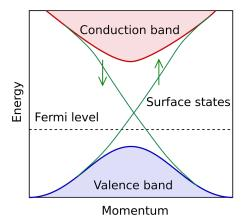
The bands (in green) of the surface states cross the Fermi level and hence are conducting. The bulk is an insulator. (Thanks to Wikipedia.)
