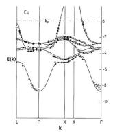
The continuous curves are estimates for copper. The dots are experimental measurements. (Thanks to Alloul for these pictures.)
